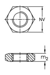
$\begin{array}{ll} m2 &= 18.0\\ Nominal size &= M36\\ NV &= 55.00\\ Thread pitch &= 2.00\\ Weight (g) &= 230.0 \end{array}$
